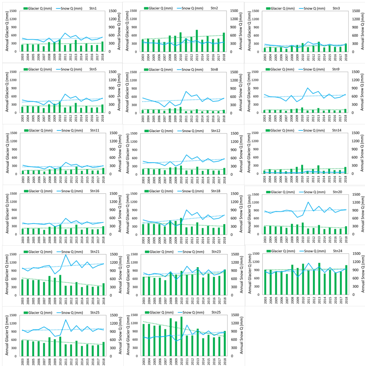
Figure 17: Annual variations and trends in Snow Q and Glacier Q across 17 stations out of 30 stations dominated with snow and glaciers during 2003-2018.
